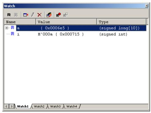
Figure 3.16 Watch window (showing a variable)
